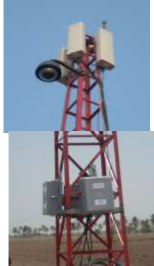
Tower with PTZ camera, Monitoring unit and Data Logger for Wireless Sensors, Wi-Fi Internet, etc.
