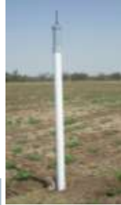
Wireless Sensor Module for Soil Moisture & Temp Sensors
